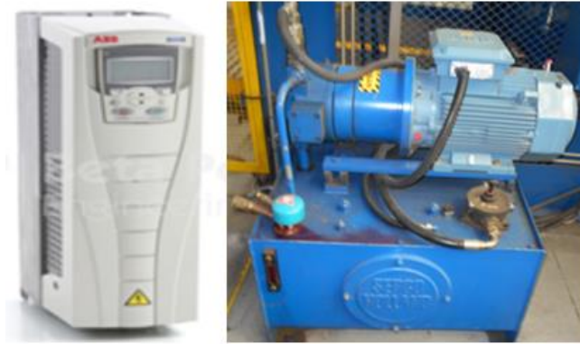
Figure 5.23 Inverter drive application on a hydraulic motor
