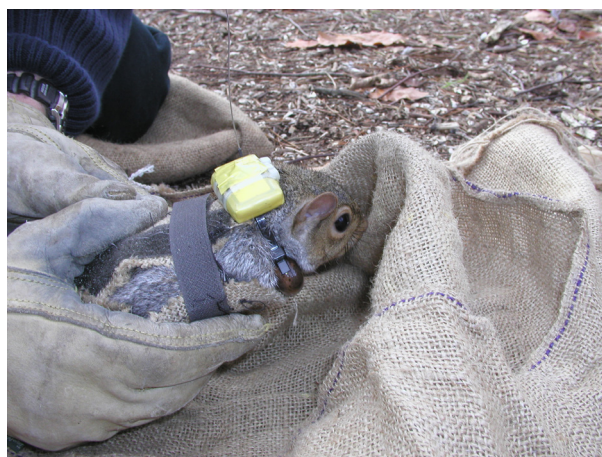
Figure 3. Fitted collar with GPS device at the top and radio transmitter underneath. Note the hessian cone with adjustable neck still to be undone, releasing the squirrel.
