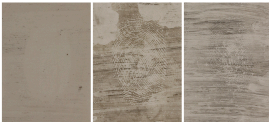
Fig. 9. Reverse development of fingerprints on ceramic using SP80/T80 surfactant at stock (left), half (middle) and quarter (right) concentrations.
