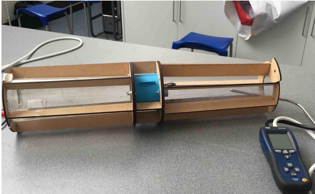
Figure 7: Image shows Manometer is connected without fixing the ends, which cause vibrations
