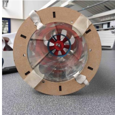
Figure 6: Image shows the Outlet view of the wind tunnel
