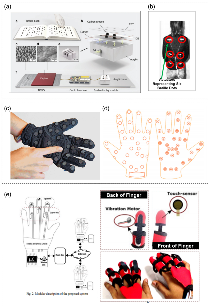
Figure 5. a) Refreshable Braille display using triboelectric nanogenerators; it enables Braille users to be able to read different English letters corresponding to the Braille code. Reproduced with permission. [123] Copyright 2021, Wiley. b) Body Braille: this device is worn on the body and has six cells to represent the different cells of standard Braille. Reproduced with permission. [127] Copyright 2008, IEEE. c) Mobile Lorm glove: introducing a communication device for deafblind people; it has fabric-based pressure sensors that enable deafblind people to compose and send messages to a remote mobile phone user. Reproduced with permission. [161] Copyright 2012, ACM. d) Mapping and position of the sensors for a smart glove developed for deafblind people who use Lorm. Reproduced with permission. [161] Copyright 2012, ACM. e) SmartFingerBraille: this glove contains touch sensors at the tip of the index, middle, and ring finger and vibrotactile actuators at the back of these fingers; the touch sensors are used to compose messages and send to a remote mobile phone user based on the Braille code. Reproduced with permission. [129] Copyright 2017, IEEE.
