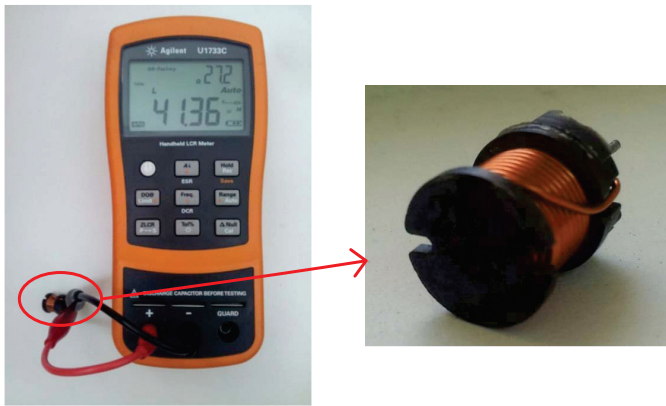
Fig. 14. Tested inductor and test value by LCR meter.
