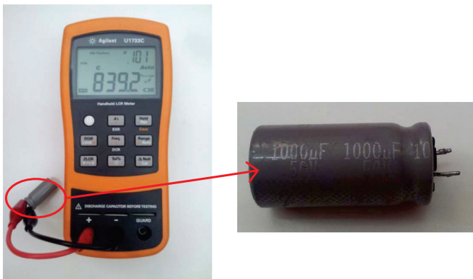
Fig. 18. Tested capacitor and test value by LCR meter.
