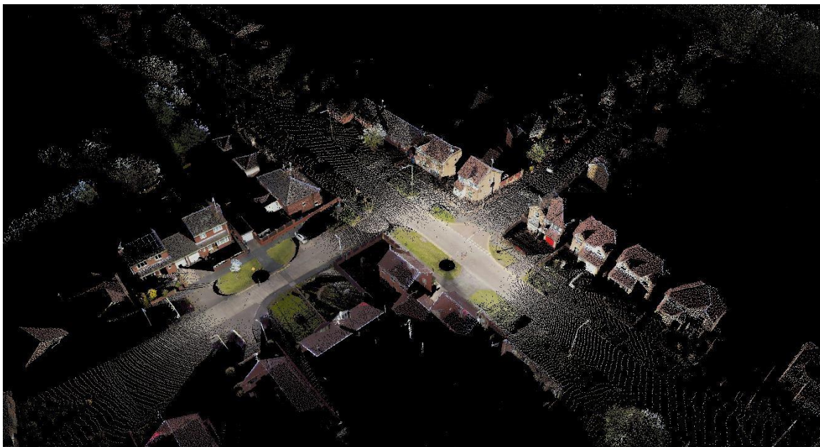
135 Figure 2. The ground LiDAR data outputs consist of a digital elevation model with colour digital 136 photographs rendered onto the digital elevation model.
