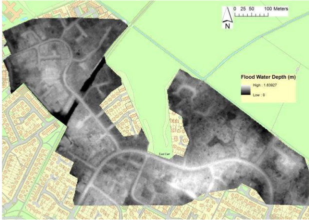
Figures 5a and 5b: Interpolated Water Depths for the 2007 2014 flood event
