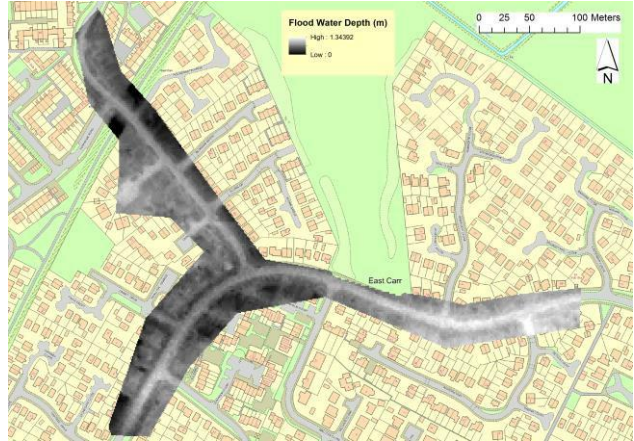
Figures 5a and 5b: Interpolated Water Depths for the 2007 2014 flood event
