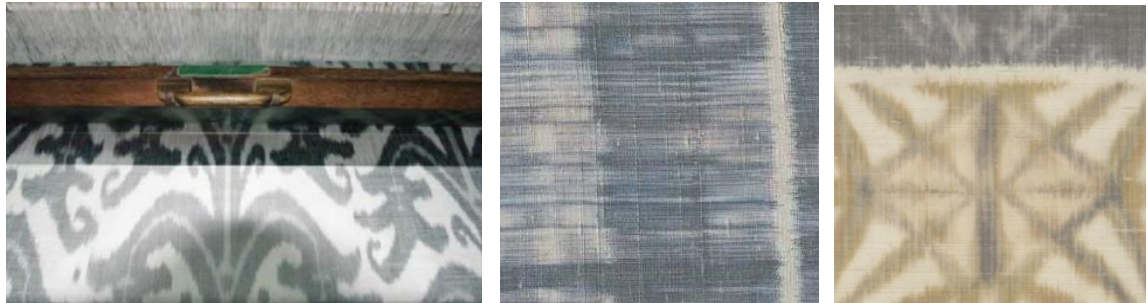
Figure 15: a. Turnbull-Designs. July 2019. Digitally Printed Warp being woven for ikat effect. b. Shibori samples. Digitally printed and woven warp. Designed by the author 2007
