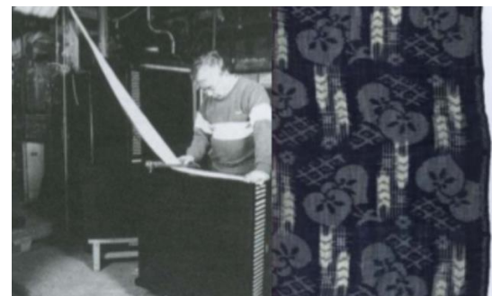
Figure 5: a. The placement of warp yarns within Itajime gasuri boards prior to dyeing. Japan. b. E-gasuri created by Itajime boards note white/grey identifying board marks on selvage. Krauss 2006
