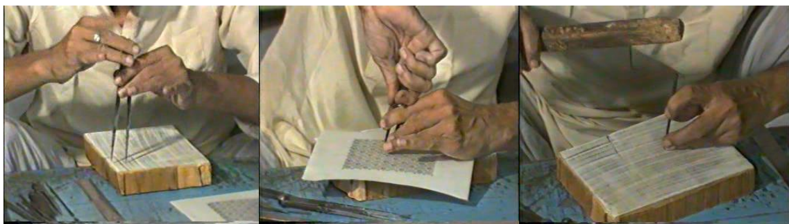
Plate-6: Drawing the design on the wood piece by making grid and taking measurement by metal stylus (Compass)
