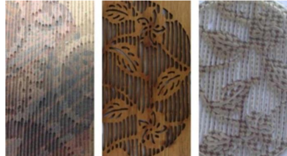
Figure 9: Digitally created clamping Boards: Jo Newton, University of Derby. 2013. a. CNC Routed MDF b. Laser-cut plywood c. Laser cut Perspex sheet
