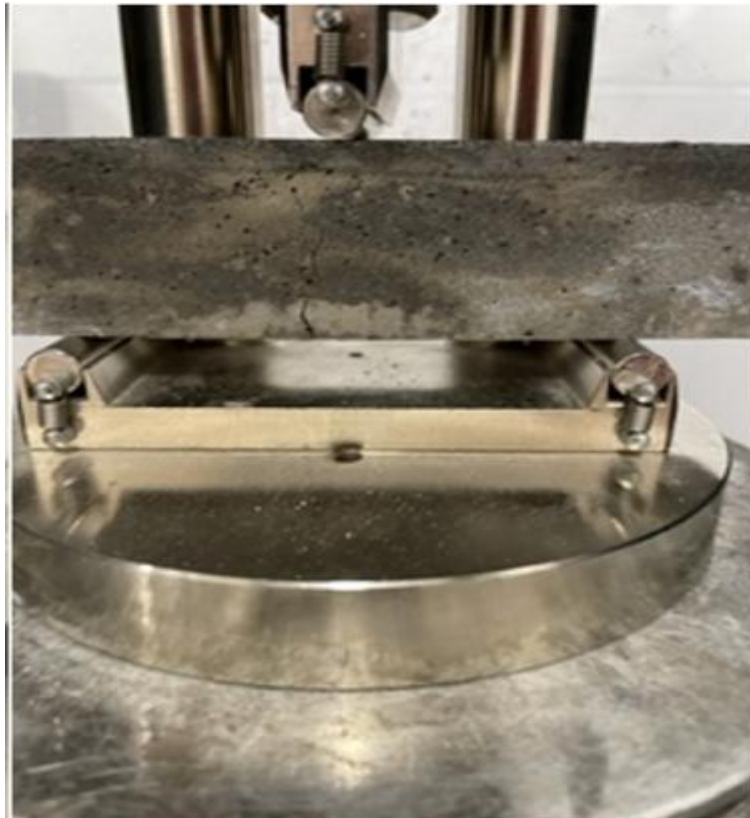
Figure 76: Three-bending testing for generating the crack.
