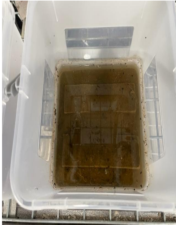
Figure 77: Prisms covered with fully saturated soil inside the containers
