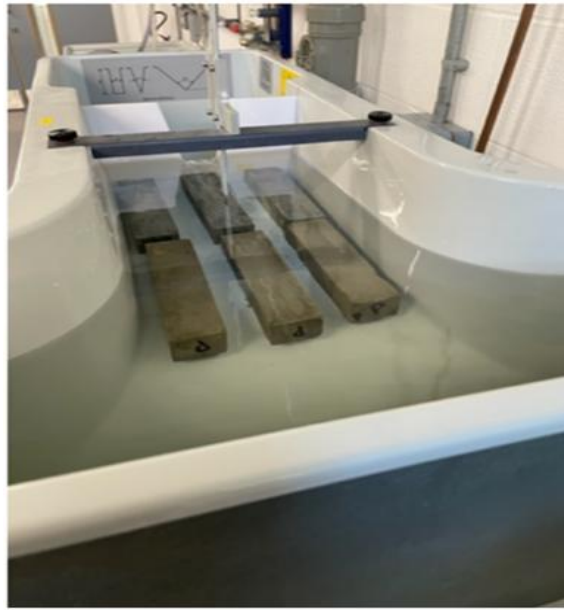
Figure 91: Digital hydraulic bench with prisms positioned within the setup.
