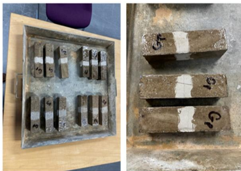
Figure 81: Mortar coating with epoxy
