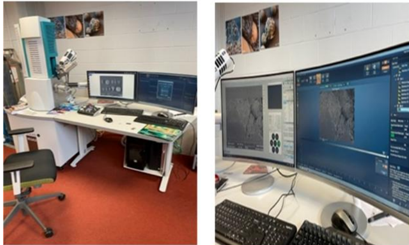
Figure 79: Scanning electron microscopy and energy dispersive X-ray (SEM-EDX).
