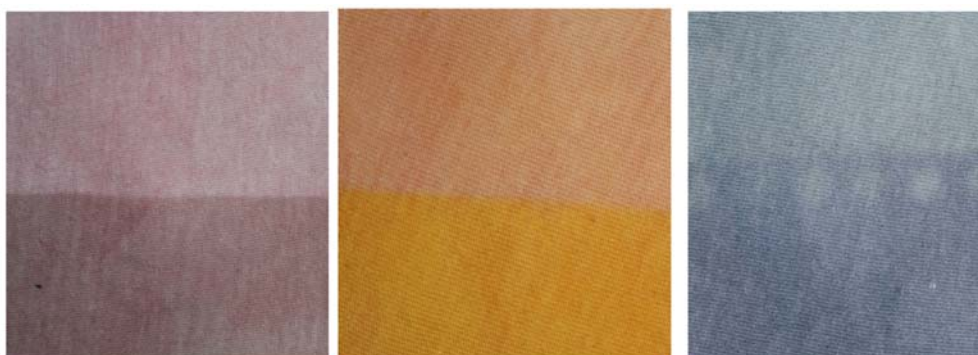
Figure 2: Fast and fugitive mixing and basic fastness testing. Madder with Blackberry, Madder with Turmeric, Woad with Blackberry
