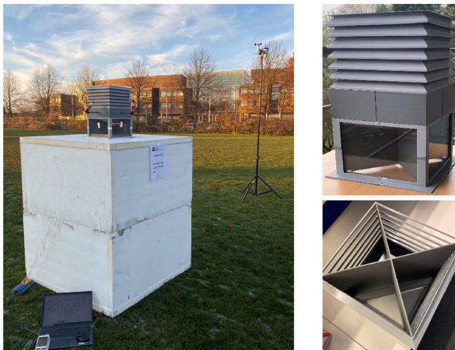
Fig. 3. The 3D-printed prototype of the windcatcher and the test room in the field test area.
