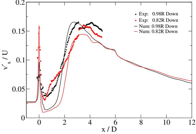
Figure 9: Streamwise rms velocity component at the vertical centre plane at two radii below the rotor axis.
