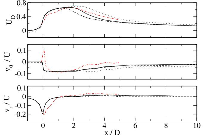
Figure 5: Streamwise velocity deficit and, tangential and radial mean velocity components at the vertical centre plane at radius  $0.82R$  below the rotor axis: LTI (dotted-lines), MTI (solid-lines), HTI (dashed-lines) and Exp. (dot-dashed-lines).
