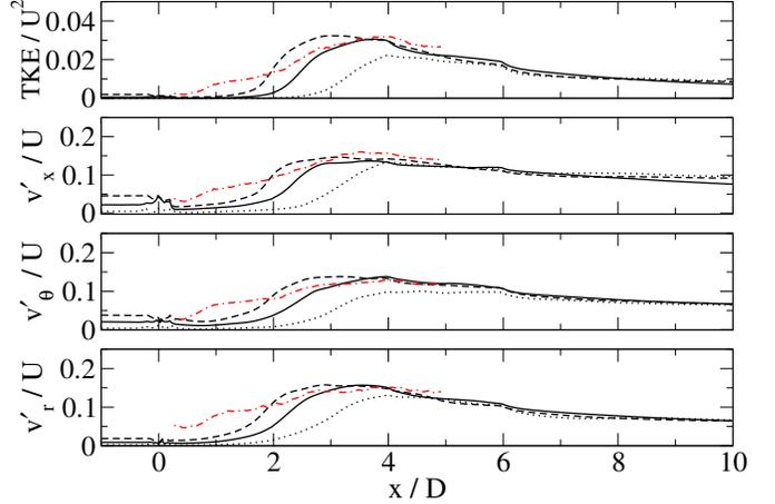
Figure 8: Turbulent kinetic energy and rms velocity components at the vertical centre plane at radius  $0.82R$  below the rotor axis: LTI (dotted-lines), MTI (solid-lines), HTI (dashed-lines) and Exp. (dot-dashed-lines).
