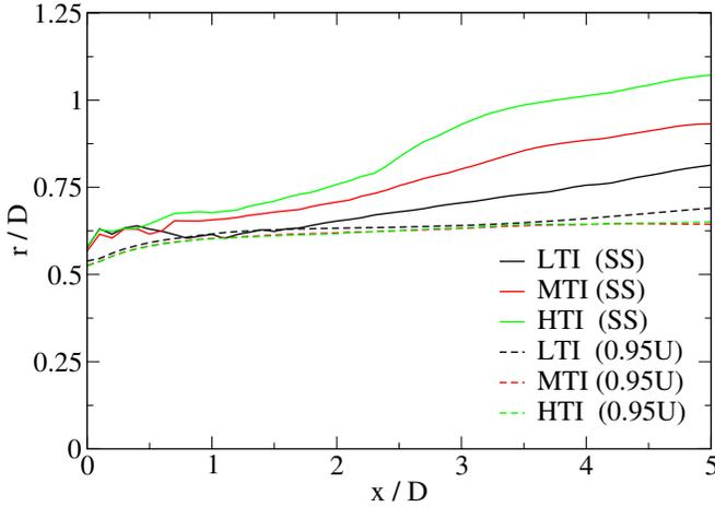
Figure 11: The upper borders of the shear layers shown in Fig. 10 (solid lines) and the wake edges calculated using  $U_{wE} = 0.95U$  (dashed lines) at the top half of the vertical centre plane.
