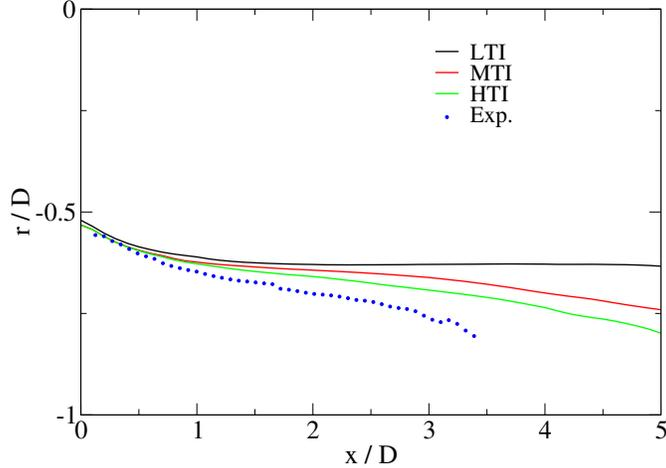
Figure 15: Wake edges calculated using  $U_{WE} = 0.95U$  at the bottom half of the vertical centre plane.
