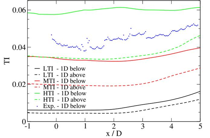
Figure 14: Turbulence intensities at the vertical centre plane below and above the rotor axis.
