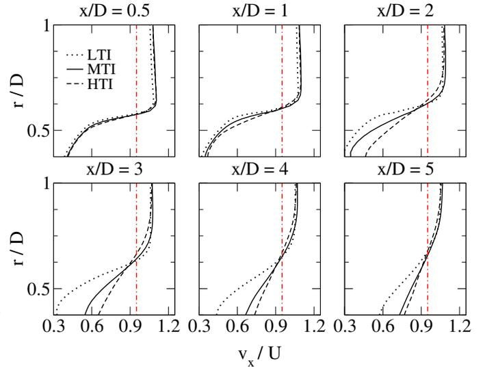
Figure 12: Streamwise mean velocity component at the top half of the vertical centre plane at different downstream locations, dot-dashed lines denote  $v_x = 0.95U$ .
