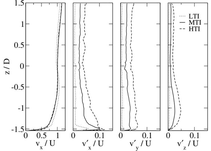
Figure 2: Streamwise mean and rms velocity components at the vertical centre plane of the channel 1D before the turbine plane.
