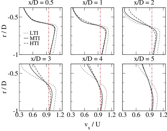
Figure 13: Streamwise mean velocity component at the bottom half of the vertical centre plane at different downstream locations, dot-dashed lines denote  $v_x = 0.95U$ .
