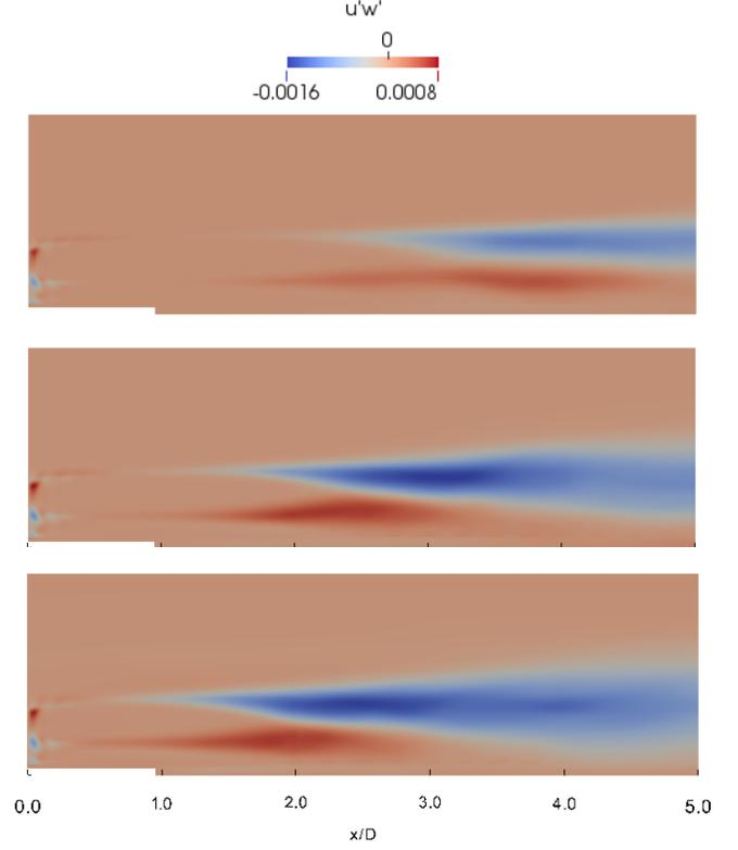
Figure 10: Shear stresses  $v'_x v'_r$  at the top half of the vertical centre plane: LTI (top), MTI (middle) and HTI (bottom).
