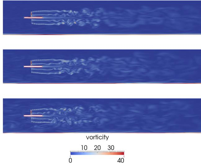
Figure 6: Vorticity at the vertical centre plane of channel for varying levels of inflow turbulence: LTI (top), MTI (middle) and HTI (bottom).
