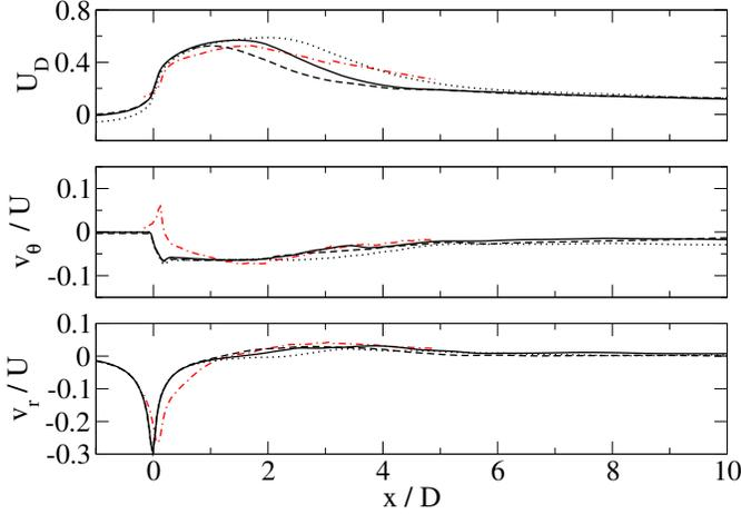
Figure 4: Streamwise velocity deficit and, tangential and radial mean velocity components at the vertical centre plane at radius  $0.98R$  below the rotor axis: LTI (dotted-lines), MTI (solid-lines), HTI (dashed-lines) and Exp. (dot-dashed-lines).
