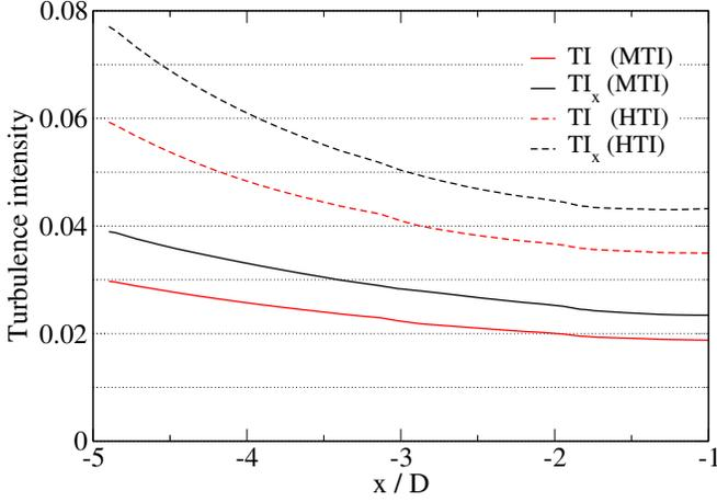
Figure 1: Downstream development of total (TI) and streamwise turbulence ( $TI_x$ ) intensities at the rotor axis height for cases MTI and HTI.
