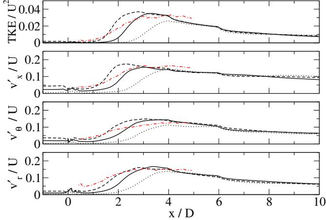
Figure 7: Turbulent kinetic energy and rms velocity components at the vertical centre plane at radius  $0.98R$  below the rotor axis: LTI (dotted-lines), MTI (solid-lines), HTI (dashed-lines) and Exp. (dot-dashed-lines).
