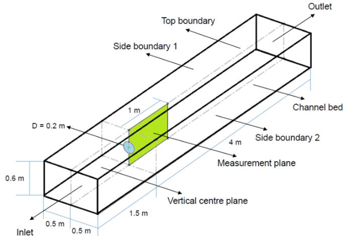
Figure 3: Schematic view of the computational domain.
