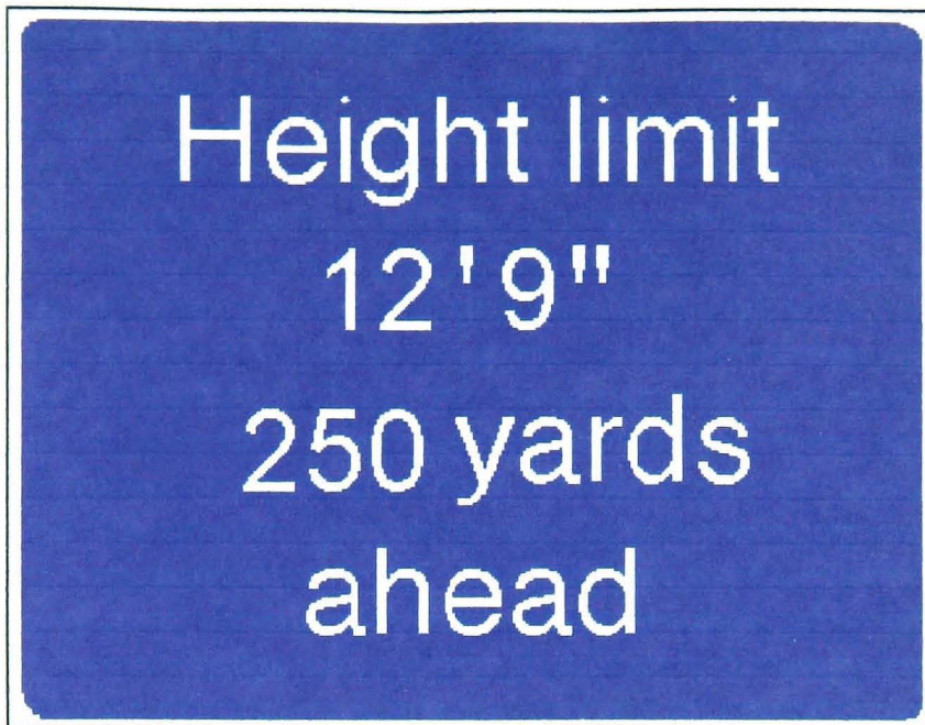
Figure 1.4: An intermediate bridge warning sign
