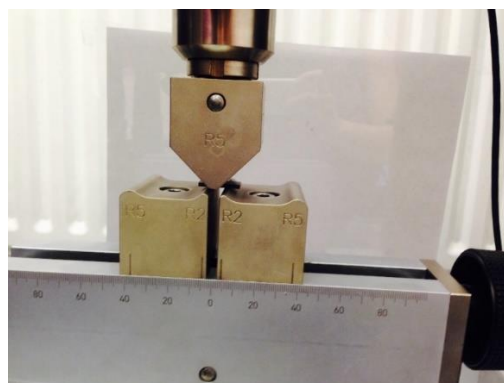
Figure 6-4 Short beam test experimental set-up (Loading roller diameter =10mm, support diameter=4mm).
