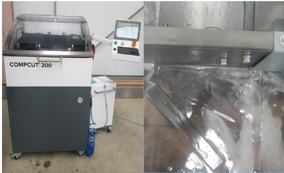
Figure 3-17 Illustration of the cutting process using COMPCUT 200.
