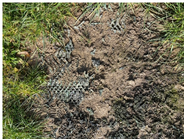
Figure 74. Evidence of plastic degradation of reinforcement matting at Timber festival site. Author's photograph.
