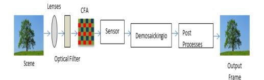
Figure 1. The digital video frame acquisition process.
