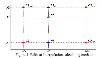
There are several equivalent ways to calculate the value of the bilinear interpolation P. An easy way to calculate the value of P would be to first calculate the value of the two blue dots, R2, and R1. R2 is effectively a weighted average of Q12 and Q22, while R1 is a weighted average of Q11 and Q21.
