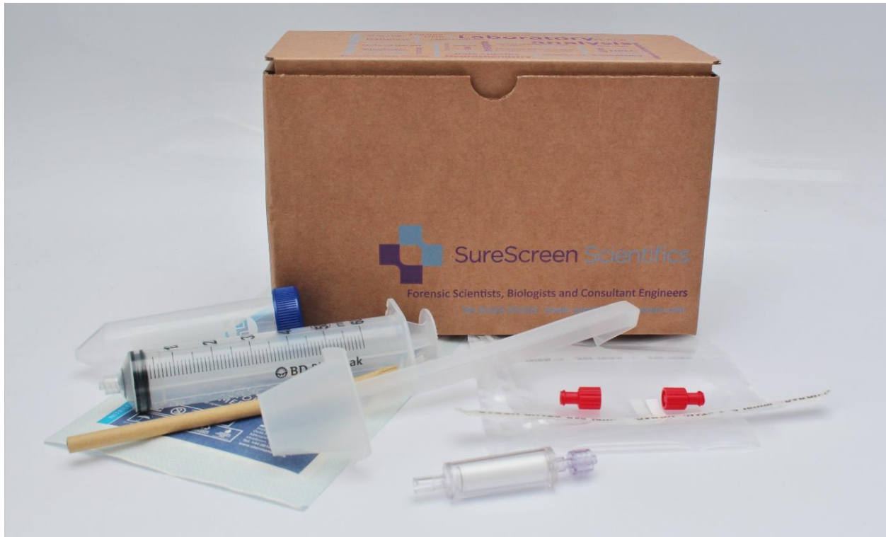
Fig. 5.14. Disposable single use kit for the Sterivex filtration eDNA sample collection method. Source author, ©Chris Troth, ©SureScreen Scientifics.
