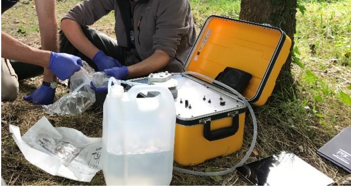
Fig. 5.5. Re-useable battery powered peristaltic pump and accessories used for the filtration sample collection approach. Source author, ©Chris Troth.
