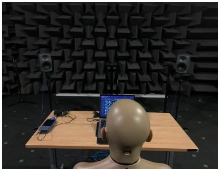
Figure 5 - A KEMAR 45BB HATS dummy head positioned to capture the BRIRs for separately capturing HRTFs representing the two loud-speaker positions.
