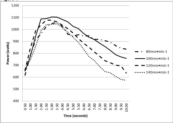
Results from 10 seconds sprint on a cycle ergometer were the cadence was restricted to 80, 100, 120 and 140revs·min<sup>-1</sup>. Graph shows mean results for all six riders' peak power and power development
