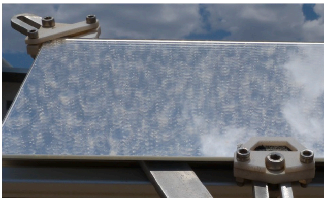
Fig. 9. Mirror surface after a strong soiling event [32].
