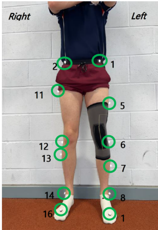
Figure 4: Anterior view of Vicon reflective markers (1 = left ASIS; 2 = right ASIS; 5 = left THI; 6; left KNE; 7 = left TIB; 8; left ANK; 10 = left TOE; 11 = right THI; 12 = right KNE; 13 = right TIB; 14 = right ANK; 16 = right TOE).
