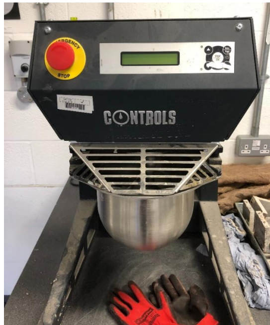
Figure 4.7: Mixer used to prepare the cement mortar specimens
