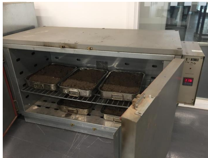
Figure 6.4: Sterilizing the soil using the oven at a temperature of 120°C
