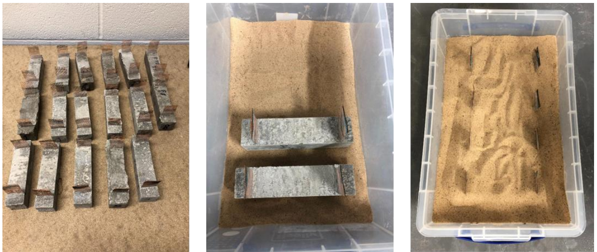
Figure 7.7: Incubation of cracked specimens within the soil
