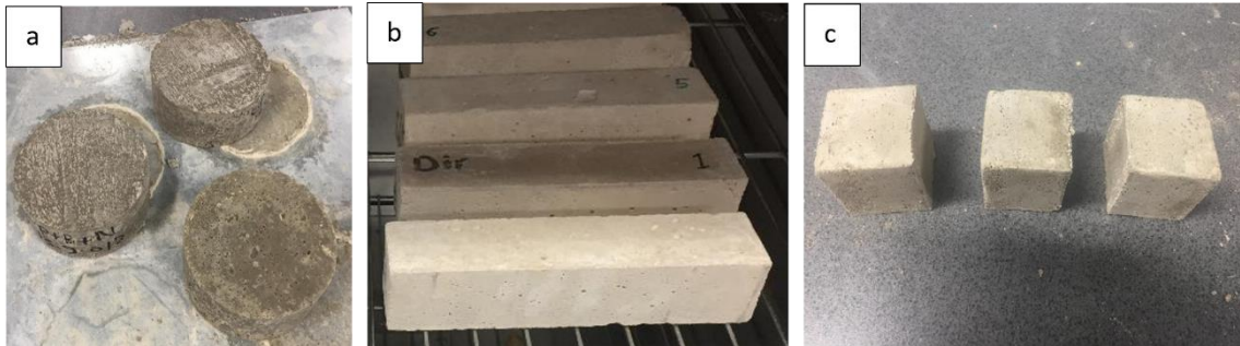
Figure 5.4: Cement mortar specimens (a) Cylindrical (b) Prisms (c) Cubes
