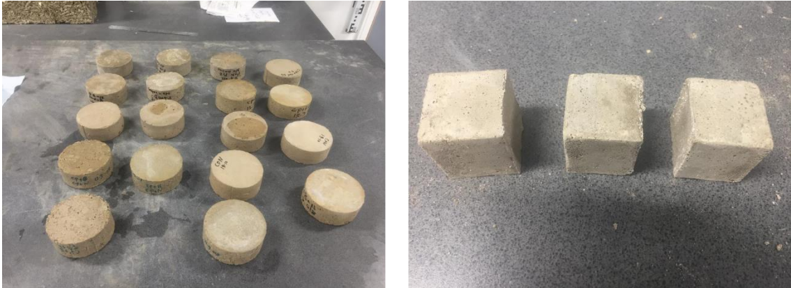
Figure 4.9: Cement mortar specimens after demoulding
