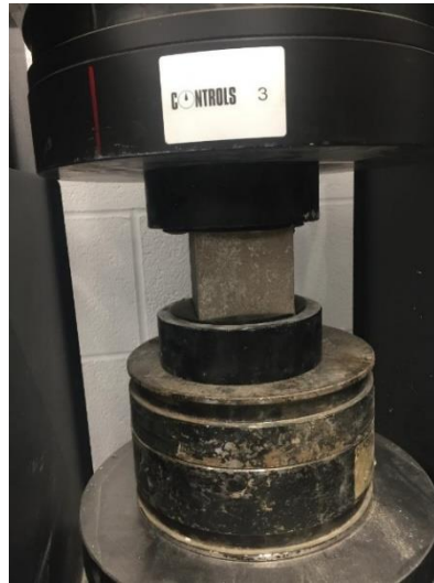
Figure 4.15: Automatic compression machine used for the compressive strength test
