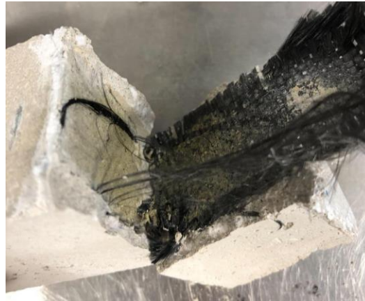
Figure 7.5: Separation of carbon fibre sheets during crack creation process
