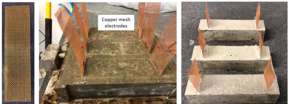
Figure 7.6: Using copper mesh electrodes with cementitious matrix
