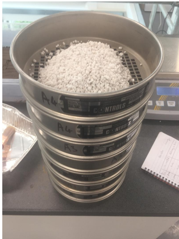
Figure 5.7: Preparation of sieves for particle size distribution test
