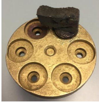
Figure 4.20: Fixing the sample on the cylindrical disc chamber
