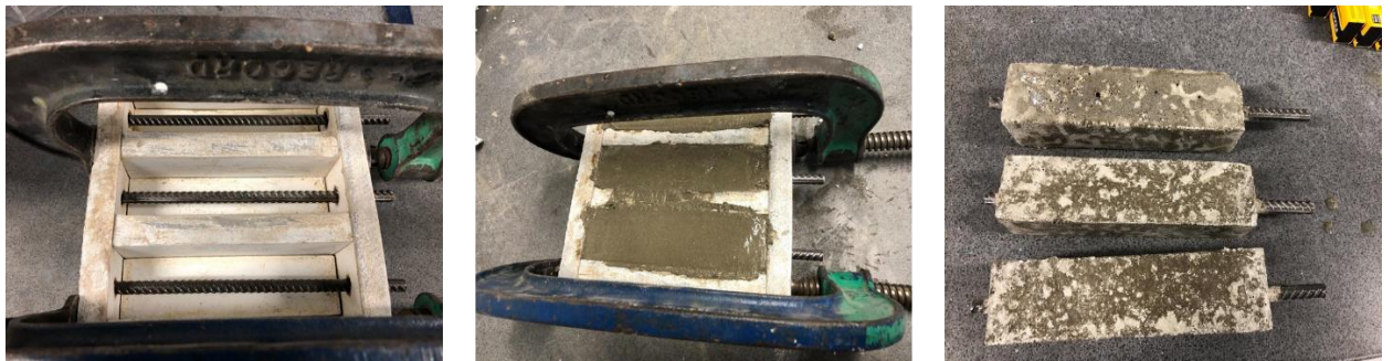
Figure 7.4: Casting of prisms mortar specimens with steel bars
