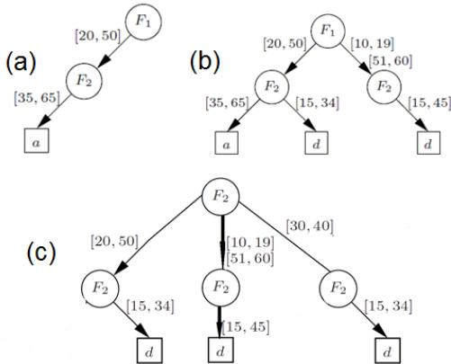
Figure 3. (a) and (b) FDD construction (c) pruning of permit space.
