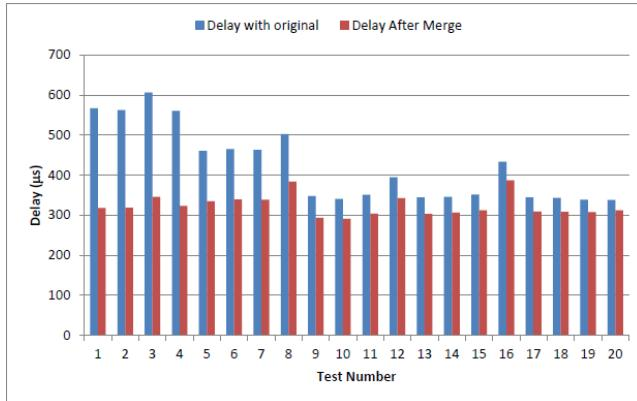
Figure 7. Packet delay for tests using real ACLs.
