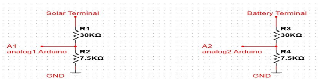
Figure C-2 Voltage Divider resistors and connection Setup
