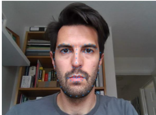
Figure 3: Webcam capture with Beyond Reality Face 68-point (blue dots) Face Tracking Overlay
