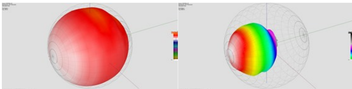
Figure 5 - JBL Control 25 attenuation balloon at 250Hz (left) and 8kHz (right)
