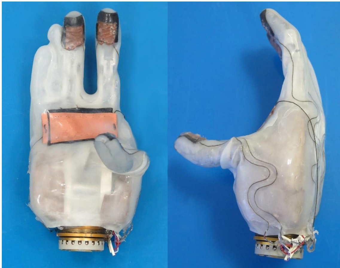
Figure 3: Silicone glove on the SNAVE hand. Sensors are on the digit tips and on the palm.
