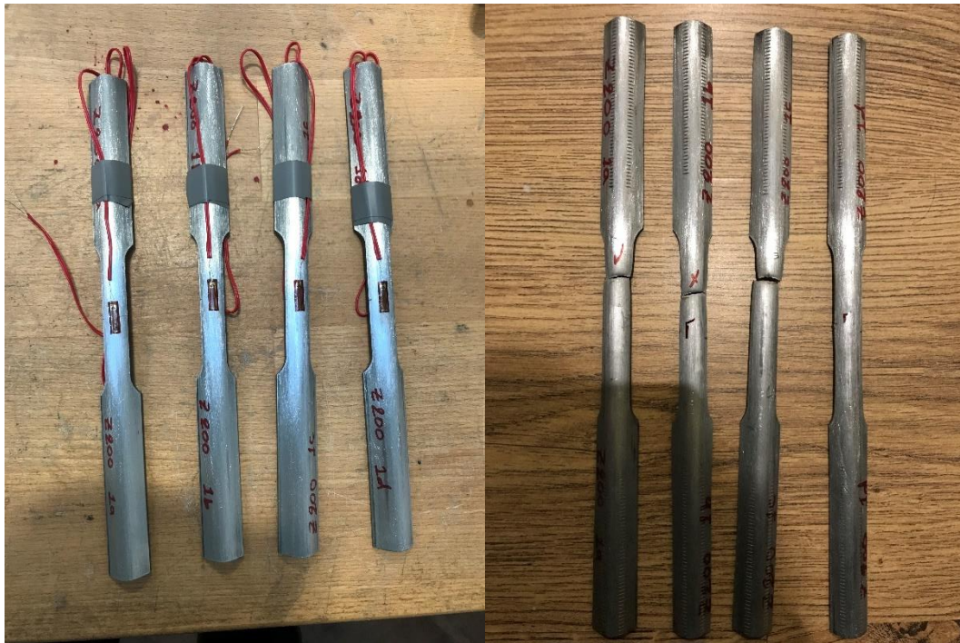
Figure 8.3. Typical tensile test setup (a) flat coupon and (b) Curved coupons
