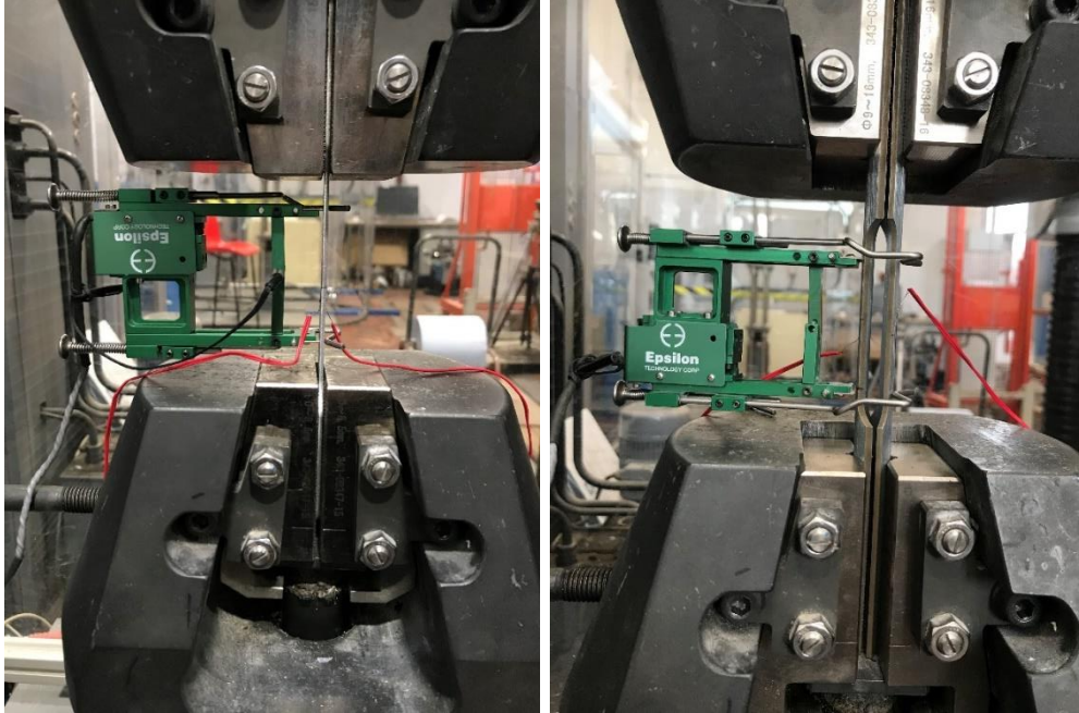
Figure 8.3. Typical tensile test setup (a) flat coupon and (b) Curved coupons
