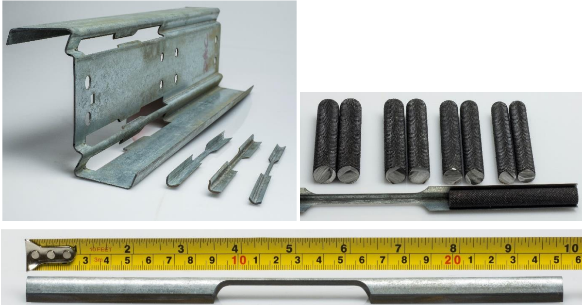
Figure 8.4. Typical curved coupons before and after testing attached with strain gauges for the cross-section Z-W200T2.0 (Extracted from curved location 1a, 1b, 1c and 1d).
