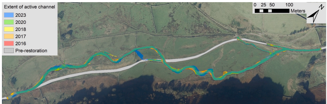
Fig. 13. Planform change at Swindale Beck following restoration. Channel extent for each year is based on low-flow, wet channel extent from orthoimages produced using UAV acquired images that were processed using SfM photogrammetry. The polygons showing the extent of the active channel are each partly transparent; where they overlay a mix of colours from different years is shown.
