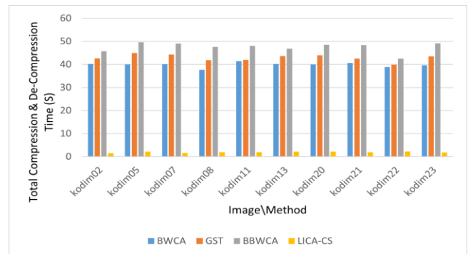
Fig. 9. Total compression and decompression time (in secs) for the proposed LICA-CS algorithm compared with state-of-the-art schemes using KODAK images
