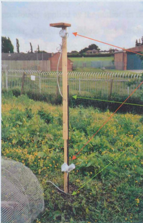
Figure 2.4: HOBO Pro Data Loggers positioned at 2 metres and 1 metres, 0.35 metres, and 10cm inside the soil.
