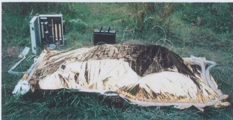
Figure 3.3: Original equipment used for the collection of volatiles showing the air entrainment kit, car battery, and the thermal blanket.
