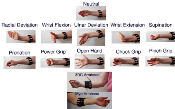
Fig. 2. The 3DC EMG datasets collection hardware and gestures included (images adopted from [5], under the Creative Commons Attribution License).
