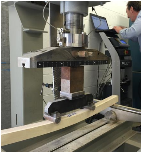
Fig. 10. Bending strength test (Source: Author)
