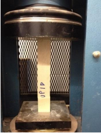
Fig. 9. Compression strength test (Source: Author)
