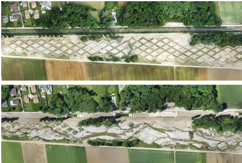
Fig. 3. Renaturation of the Aire River – construction of a channel/landscape architecture – Aerial view showing evolution between June 2014 and May 2015. Courtesy © Superpositions.
