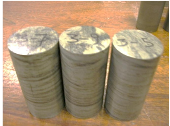
Figure 3. Intact samples of the muddy siltstone.
