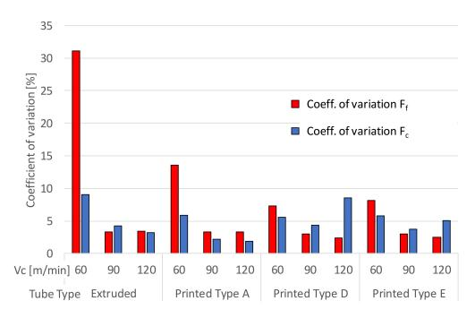
Figure 9. Coefficient of variation (Fc and Ff), for the extruded and AM tube samples.
