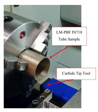
Figure 3. Experimental setup for machining.
