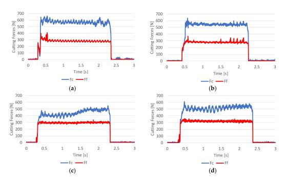
**Figure 6.** Cutting forces evolution ( $F_c$  in blue,  $F_f$  in red) for the tested tubes at a cutting speed of 120 m/min: (**a**) Extruded tube, (**b**) AM tube A, (**c**) AM tube D, (**d**) AM tube E.
