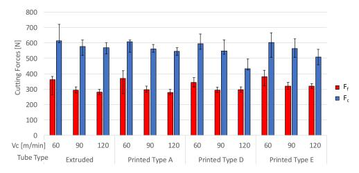
**Figure 5.** Average cutting forces (F<sub>c</sub> and F<sub>f</sub>) for the extruded and AM tube samples A, D, and E with a variation in Vc.
