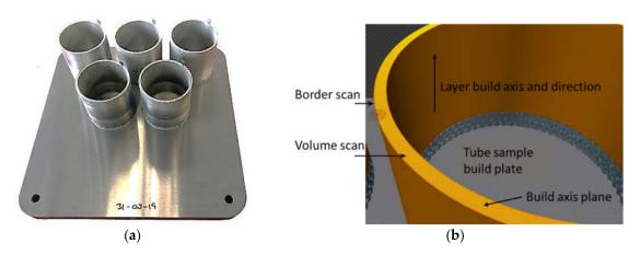
**Figure 2.** Additive manufacturing (AM) fabricated tube samples in the Renishaw AM250 SLM machine (**a**), and tube sample build orientation definitions (**b**).
