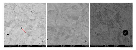
Figure 4. SEM images of spherical porosity in tube samples: (a) Tube A, (b) Tube D, (c) Tube E.
