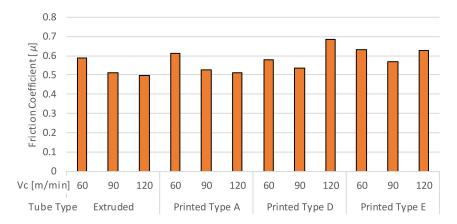
Figure 8. Mean coefficient of friction for the extruded and AM tube samples.
