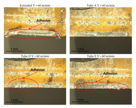
**Figure 10.** Rake face of the tool tip used for machining the extruded and the AM tubes with Vc at 60 m/min.
