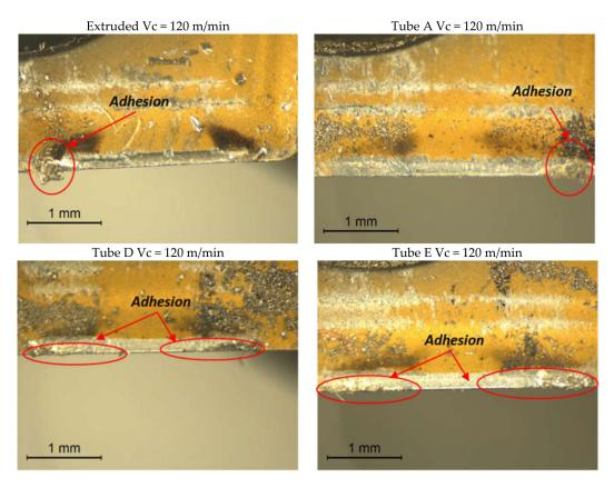
**Figure 7.** Rake face of the cutting tool tip used for machining the extruded and the AM tubes with Vc at 120 m/min.
