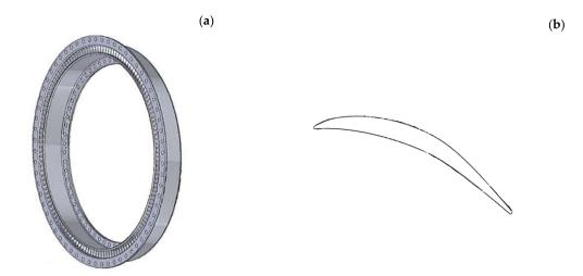
**Figure 1.** (a) Outlet guide vane 605 mm outside diameter; (b) mid-section geometry of NACA-6 series airfoil of the outlet guide vane.
