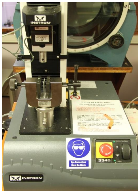
Figure 3: The Instron tensile testing machine
