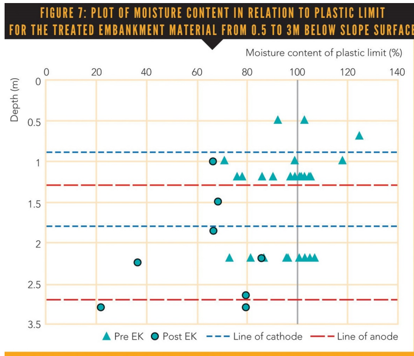
Figure 7 shows the pre-treatment moisture contents lay at or around the corresponding plastic limits, whereas the post-treatment data indicates that the EK treatment reduced the moisture content well below the plastic limit. The reduction in soil plasticity is associated with physio-chemical changes in the soil including cementation, precipitation, and flocculation effects which act together with consolidation and shear strength improvement, (Milligan, 1994; Pugh 2002). Statistical analysis carried out on the data shown in figures 6 and 7 is shown in table 4. The reduction in natural moisture confirms the discharge of water observed during the active treatment period (figure 4).
