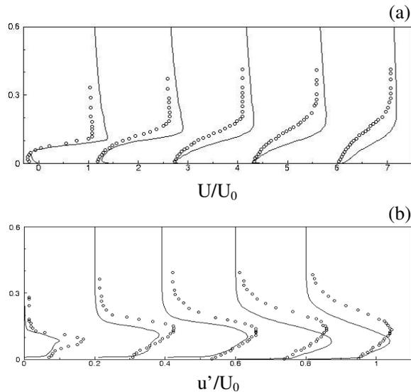
Fig. 3 Mean axial velocity and r.m.s profiles at five axial locations measured from the leading edge for the blunt leading edge case. Left to right,  $x/x_R = 0.2, 0.4, 0.6, 0.8, 1.0$ . Solid line, LES; symbols, experimental data.
