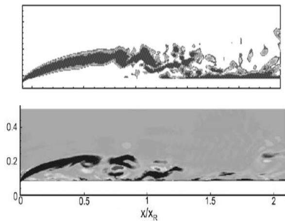
Fig. 4 Instantaneous spanwise vorticity in the  $(x, y)$  plane, above: smooth leading edge; below: blunt leading edge.
