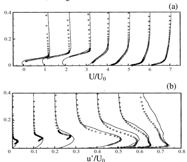
Fig. 2 Mean axial velocity and r.m.s profiles at seven axial locations measured from the blend point for the smooth leading edge case. Left to right,  $x/x_R = 0.22, 0.44, 0.66, 1.09, 1.64, 2.55$ . Solid line, LES; symbols, experimental data.
