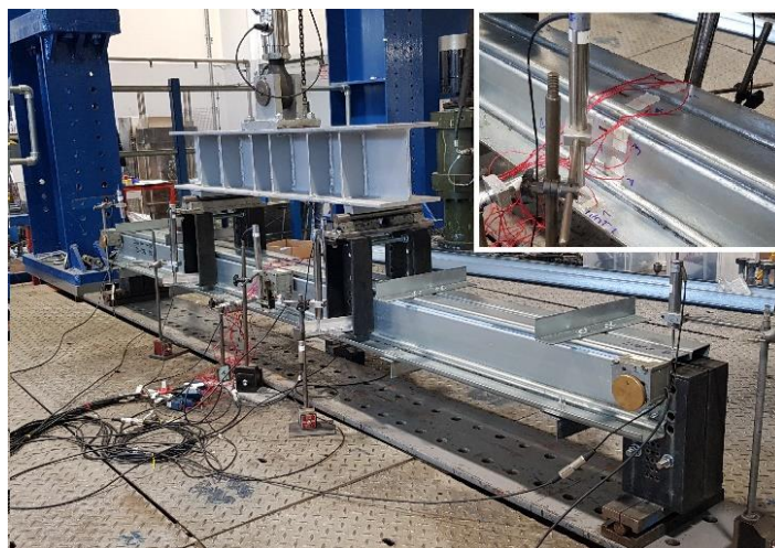
Figure 3: Four-point bending test setup, showing zed sections and strain gauge and LVDTs arrangement at mid-span of the sections (in the small box).
