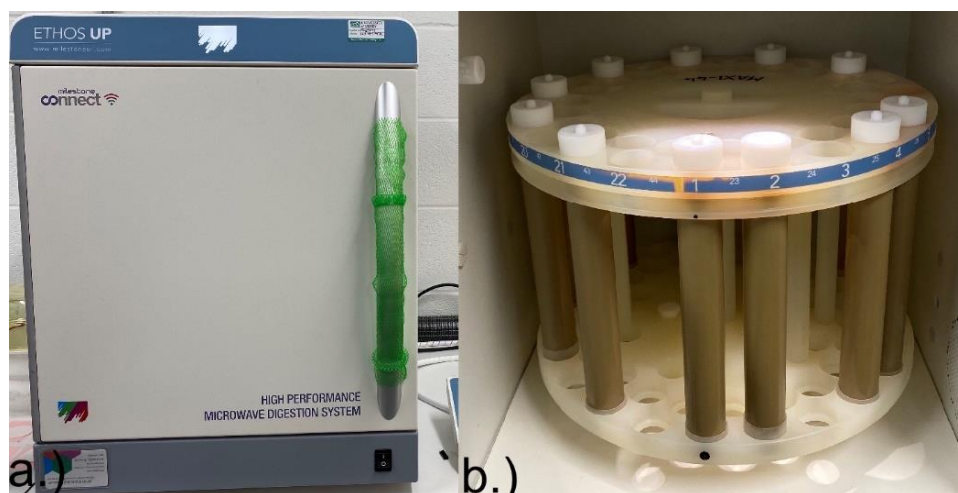
Figure 3.6 a.) High performance microwave digestion system, b.) tubes containing samples.
