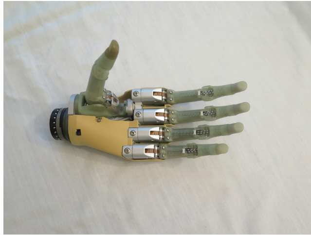
Figure 5. The i-limb has five independently powered digits, controlled by a traditional myoelectric system (image source: David Foord, 2008)
