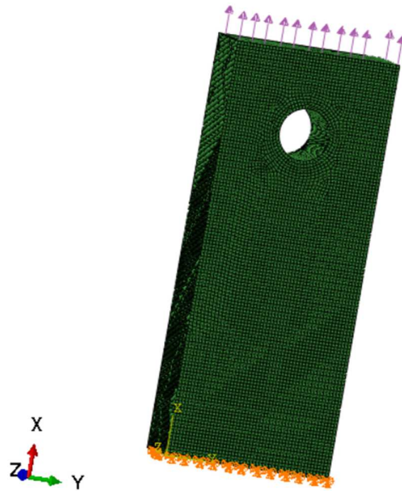
Figure 10. The applied load as a negative pressure. The orange symbol is a representation of the Boundary Condition in Abaqus 6.14. The arrow is a graphic representation of the load.
