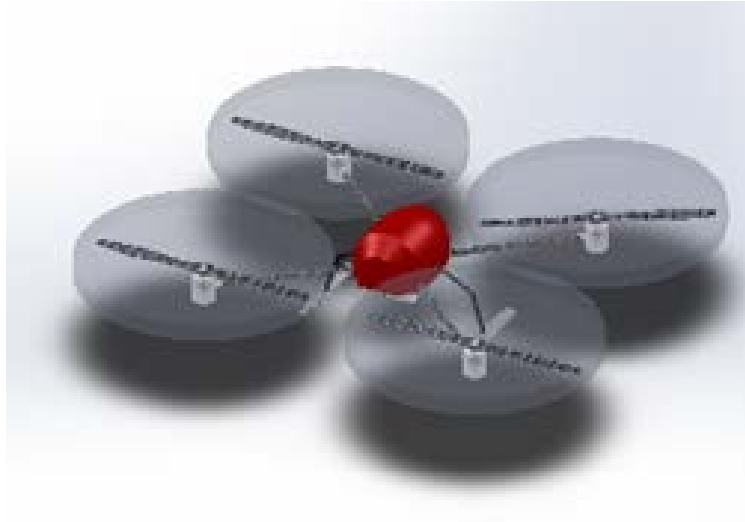
Figure 5-4: SolidWorks 3-D model of the quad-rotor helicopter
